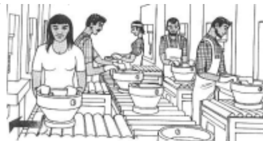
A passive conveyor line at working height
