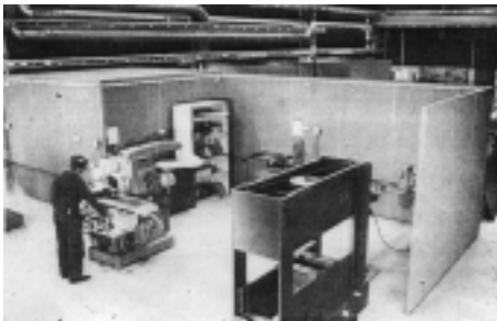
Acoustic screens (courtesy of Ecomax Acoustics Ltd.)
