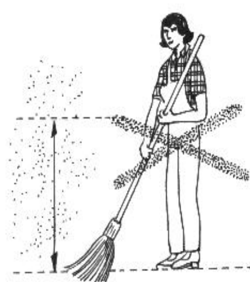
It will take a full working day before all the small dust particles have fallen to the ground. That's why the use of vacuum cleaning is strongly recommended.
