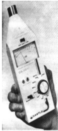
A hand held sound meter allows you to know how loud the noise is and what 'dose' a worker gets each day.
